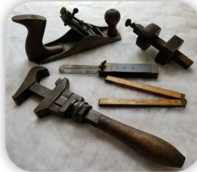
Carpenter's tools owned by John H. Minnich used during his time living in the historic Royer House at the turn of the 20th Century. Clockwise from left: Plane, adjustable scribe, sliding bevel square monogrammed "J.H.M.", foldable ruler, and pipe wrench. (Given in memory of donor's father, Emory C. Minnich)
